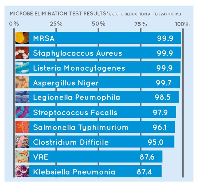
\*In an independent lab test, 10 common microbes were selected, and each of them was incubated on panels for 24hrs at 98.6 °F and >90 RH. As the table shows, AM-Clad panels demonstrate high antimicrobial activity. Use of AM-Clad, along with an adequate cleaning regime, would significantly reduce microbial growth, including dangerous pathogens.
